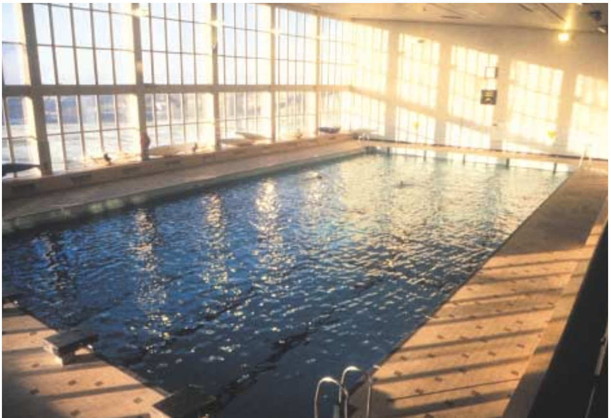
If not treated with care, the introduction of natural light can cause problems of reflection and glare.
